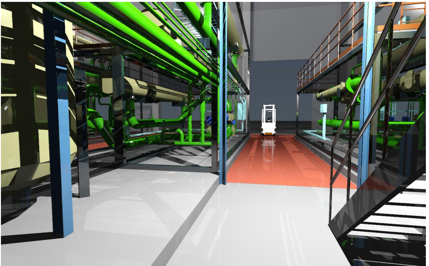
Above: Enviro's design of a pyrolysis plant with a capacity of 30,000 tons tyres/year and 9,000 tons of recovered Carbon Black
